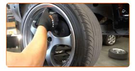
Remove the wheel hub nut cap. Use a crowbar. Use a hammer.
