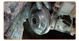
Unscrew the fasteners of the water pump housing. Use a drive socket #10. Use a ratchet wrench.
