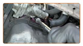
Remove the thermostat housing.
