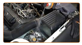
Loosen the fuel filter mounting. Use a drive socket #13. Use a ratchet wrench.
