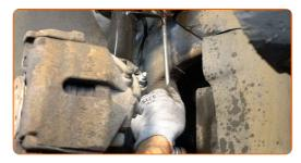
Tighten the fastener connecting the stabilizer link to the stabilizer bar. Use a combination spanner #18. Use a drive socket #18. Use a torque wrench. Tighten it to 65 Nm torque.
