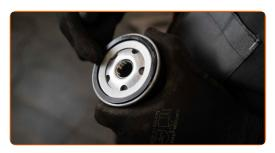
Screw the new filter into its place. Use the 76/14-F socket. Observe the recommended tightening torque.
