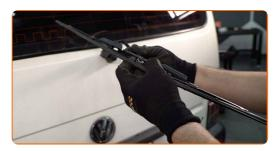
Replacement: windshield wipers – VW Fox Hatchback (5Z1, 5Z3, 5Z4). Tip from AUTODOC:
