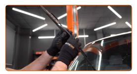
Turn the wiper blade by ninety degrees. Remove the blade from the wiper arm.
