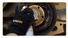
17 Install the brake drum and fasten it.
