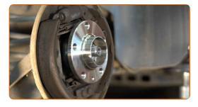
Tighten the hub. Use drive 12-point socket #30. Use a torque wrench. Tighten it to 175 nm torque.
