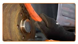
Treat the contacting surface. Use copper grease.
