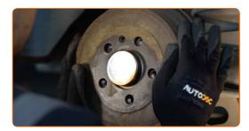
Tigten the brake drum fasteners. Use a Phillips screwdriver. Use a torque wrench. Tighten it to 4 Nm torque.
