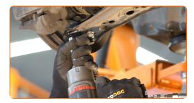
p Disconnect the spherical joint from the arm.
