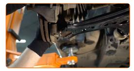
Screw the fasteners of the ball joint. Use a drive socket #13. Use a ratchet wrench.
