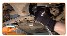
Unscrew the fastener connecting the ball joint to the suspension control arm. Use a drive socket #13. Use a tap wrench.
