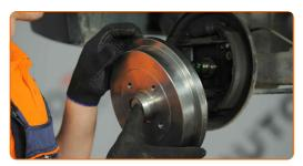
Replacement: brake shoes – VW Fox Hatchback (5Z1, 5Z3, 5Z4). Tip:
