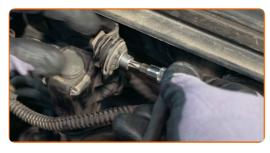
6 Unscrew the brake fluid reservoir cap.
