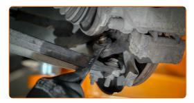
Loosen the fastening nut, remove the arm from the steering knuckle using a ball joint puller. If necessary, use a crowbar.
