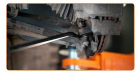
Unscrew the front arm fastener. Use a drive socket No.18 or ring spanner No.18.
