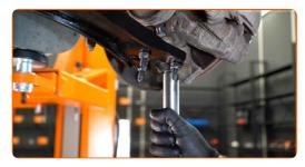
Screw the front arm fastener. Use a drive socket No.18 or ring spanner No.18. Tighten it to 70 Nm torque.+90°
