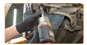
Disconnect the spherical joint from the arm.
