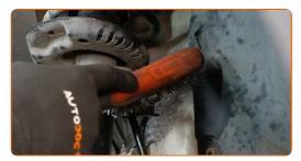
Unscrew the fastener connecting the stabilizer link to the shock strut. Use a drive socket #19. Use a ratchet wrench.
