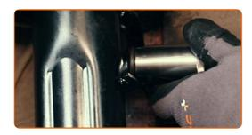
Unscrew the fastener connecting the stabilizer link to the stabilizer bar. Use a combination spanner #18. Use XZN #6. Use a ratchet wrench.
