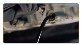
Replacement: engine oil and filter – VW Derby II (86C, 80). Tip from AUTODOC:
