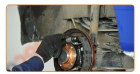
Screw the brake cylinder fastening bolts. Use Torx T30. Use a torque wrench. Tighten it to 8 nm torque.
