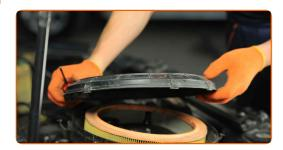
6 Remove the filter element from the filter housing.
