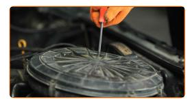
Release the air filter cover clips.
