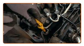
6 Clean the oil filter housing cap. Use all-purpose cleaning spray.
