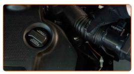
Fasten the clamp on the air intake hose. Use water pump pliers.
