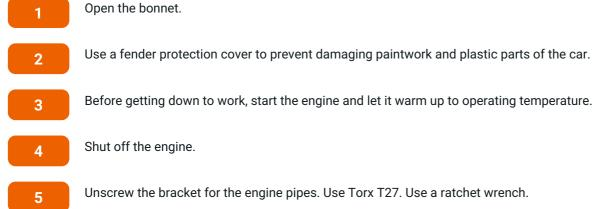
Unscrew the bracket for the engine pipes. Use Torx T27. Use a ratchet wrench.
