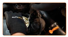
Remove the o-rings. Use a flat screwdriver.
