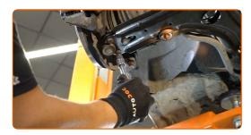
Treat the shock strut fasteners. Treat the fasteners of the ball joint. Treat the fastener connecting the tie rod end to the steering knuckle. Use copper grease.
