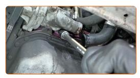
Remove the thermostat housing.
