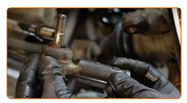
Clean the mounting seats of the tie rod end. Use a wire brush. Use all-purpose cleaning spray.
