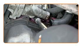
Remove the thermostat housing.
