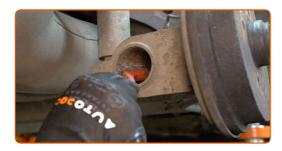
Unscrew the lower fastener connecting the shock strut to the steering knuckle. Use a combination spanner #17. Use a drive socket #17. Use a tap wrench.
