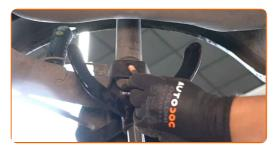
Screw in the lower fastener of the shock strut. Use a combination spanner #17. Use a drive socket #17. Use a tap wrench.
