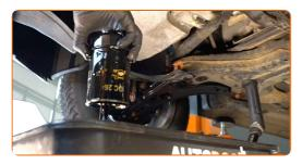
Replacement: engine oil and filter – VW Corrado (53i). Tip from AUTODOC experts:
