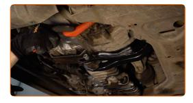
Put a waste oil container with at least 3 l capacity under the drainage hole.
