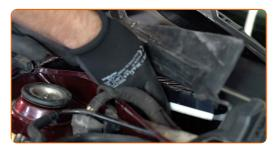
Remove the cabin air filter housing.
