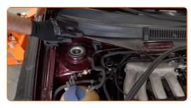
13 Install the upper seal on the firewall.
