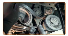
Return the tensioner pulley to its initial position. Use a combination spanner #16.
