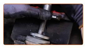
18 Install the brake caliper guide pins.
