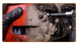
Tighten the brake caliper fasteners. Use HEX No.H7. Use a torque wrench. Tighten it to 30 nm torque.
