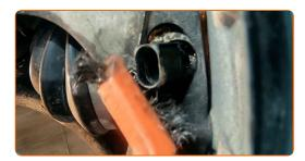
8 Unscrew the ABS sensor fastener. Use HEX No.H5. Use a ratchet wrench.
