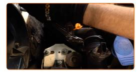
Release the air filter cover clips.
