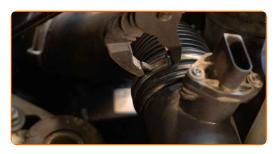
Attach the power steering reservoir.
