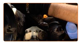
Release the air filter cover clips.
