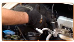
Remove the cabin air filter housing.
