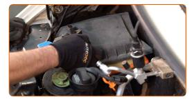
Press the air filter cover clips into place.
