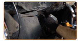
Unscrew the filter housing fastening bolts. Use HEX No.H5.
