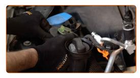
Loosen the clamp and remove the intake air hose from the filter housing. Use water pump pliers.
