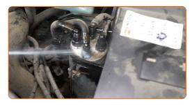
Disconnect the fuel supply lines from the fuel filter. Use a flat screwdriver.
