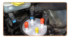
Screw in the fuel filter mounting bracket. Use a drive socket #10. Use a ratchet wrench.
