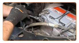
Screw in the fasteners of the back section of the engine cover. Use a flat screwdriver.
