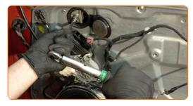
Install the covers on the window raiser fasteners.
