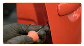
Install the cover on the exterior door handle fastener.
