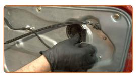
Attach the mirror adjuster connector to the control unit.
