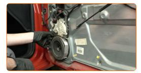
43 Attach the wiring harness to the protective cover of the door.
