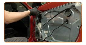
Tighten the door lock fasteners. Use XZN #8. Use a torque wrench. Tighten it to 20 nm torque.
