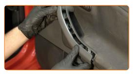
Screw in the door card fasteners. Use a Phillips screwdriver.
