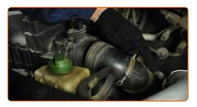
6 Release the air filter cover clips.
