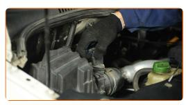
Detach the air intake hose clamp. Use clic-R collar pliers.
