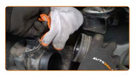
Reinstall the air filter cover. Fasten it.
