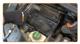
Replacement: air filter – VW California T6 Minibus (SGC, SGG, SHC). Tip from AUTODOC experts:
