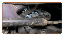
Replacement: serpentine belt – VW California T5 Minibus (7EC, 7EF, 7EG, 7HF). Tip from AUTODOC:
