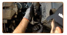
Replacement: anti roll bar links – VW Caddy V Kombi (SBB, SBJ). Tip from AUTODOC:
