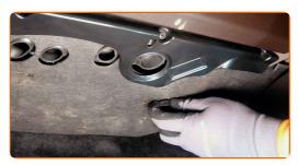
Remove the bottom cover of the glove box.
