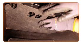
Screw in the fasteners of the bottom trim panel.
