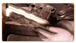
Install the bottom cover of the glove box.
