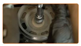
Remove the crankshaft pulley.
