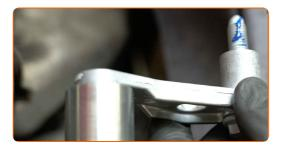
Install the timing belt idler pulley bracket with integrated pulley.
