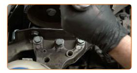
Remove the support from under the engine.
