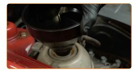
Pour coolant in the coolant reservoir.
