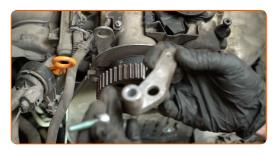
Make a mark on the camshaft gear. Make a mark on the timing belt.
