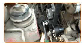
Remove the camshaft gear locking tool.
