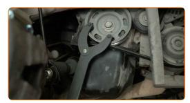
799 Tighten the crankshaft pulley fastener. Use 12-point socket No.21. Use a torque wrench. Tighten it to 90 Nm torque.+90°
