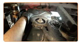
Tighten the fasteners of the lower timing cover. Use a drive socket #10. Use a torque wrench. Tighten it to 8 Nm torque.
