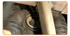
Remove the serpentine belt tensioner pulley.
