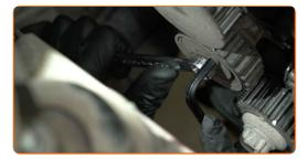
Remove the timing belt tensioner pulley.
