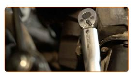
Unscrew the crankshaft pulley fastener. Use 12-point socket No.21. Use a ratchet wrench.
