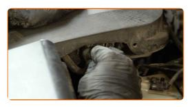
109 Remove the coolant reservoir cap.
