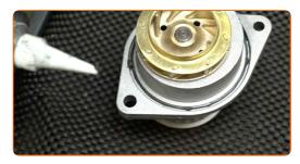
Install the water pump gasket.
