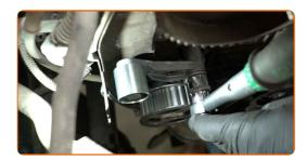
Adjust the timing belt tension by moving the tensioner pulley. Use a combination spanner #16. Use HEX No.H6.
