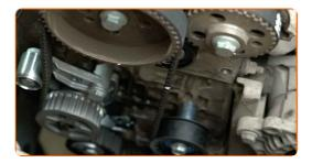
Replacement: water pump + timing belt kit – VW Caddy III Van (2KA, 2KH, 2CA, 2CH). Tip:
