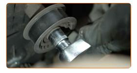
Remove the timing belt idler pulley from its mounting seat.
