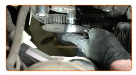
Remove the timing belt idler pulley bracket with integrated pulley.
