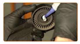
Install the serpentine belt tensioner pulley.
