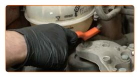
Detach the coolant pipe bracket.
