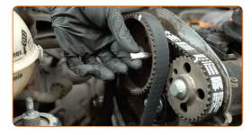
Turn the crankshaft pulley. Use 12-point socket No.21. Use a ratchet wrench.
