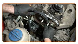
Replacement: water pump + timing belt kit – VW Caddy III Van (2KA, 2KH, 2CA, 2CH). AUTODOC recommends:
