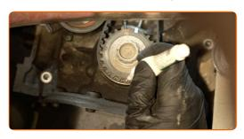
Make a mark on the camshaft gear.
