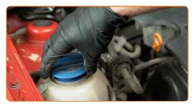
Screw on the coolant reservoir cap.
