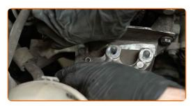
Screw in the upper fasteners of the engine mount. Use a drive socket #16. Use a ratchet wrench.
