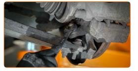
Loosen the fastening nut, remove the arm from the steering knuckle using a ball joint puller. If necessary, use a crowbar.
