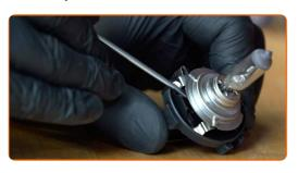
Replacement: headlight bulb – VW Caddy III Van (2KA, 2KH, 2CA, 2CH).
