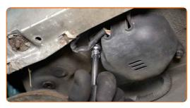
Remove the oxygen sensor housing cover.
