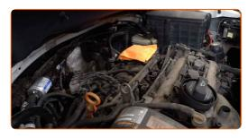
Detach the crankcase ventilation hose from the oil filler neck.
