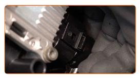
Connect the spark plug wires to the ignition coil.
