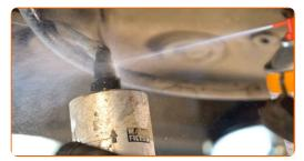
Disconnect the fuel supply lines from the fuel filter. Use a crowbar.
