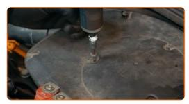
Remove the air filter housing.
