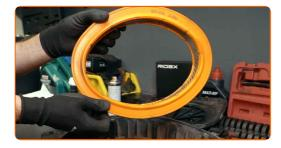
Clean the air filter cover and housing. Use all-purpose cleaning spray.
