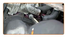
9 Remove the thermostat housing.
