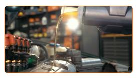
Replacement: engine oil and filter – VW Caddy II Pickup (9U7). Professionals recommend:
